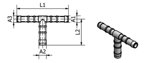
Ext. Hose Diameter A3 = 8 Ext. Hose Diameter A1 = 8 Ext. Hose Diameter A2 = 8 L1 = 58 L2 = 30
